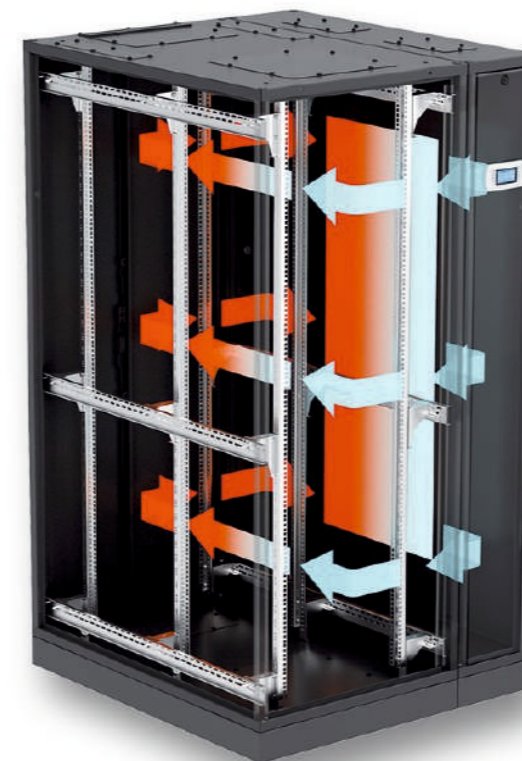
Server cabinet with a side heat exchanger. Cabinet width: 800 mm, heat exchanger width: 300 mm. Cabinet door with mineral safety glass
